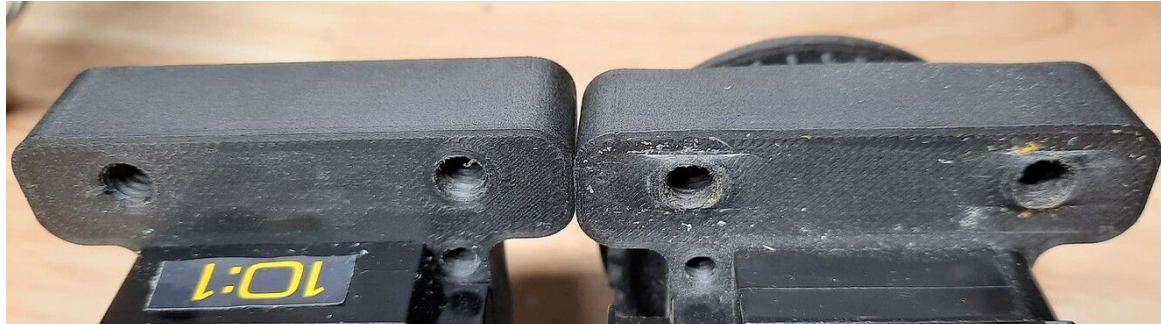
Plastic creep example - new (left) vs used (right)
